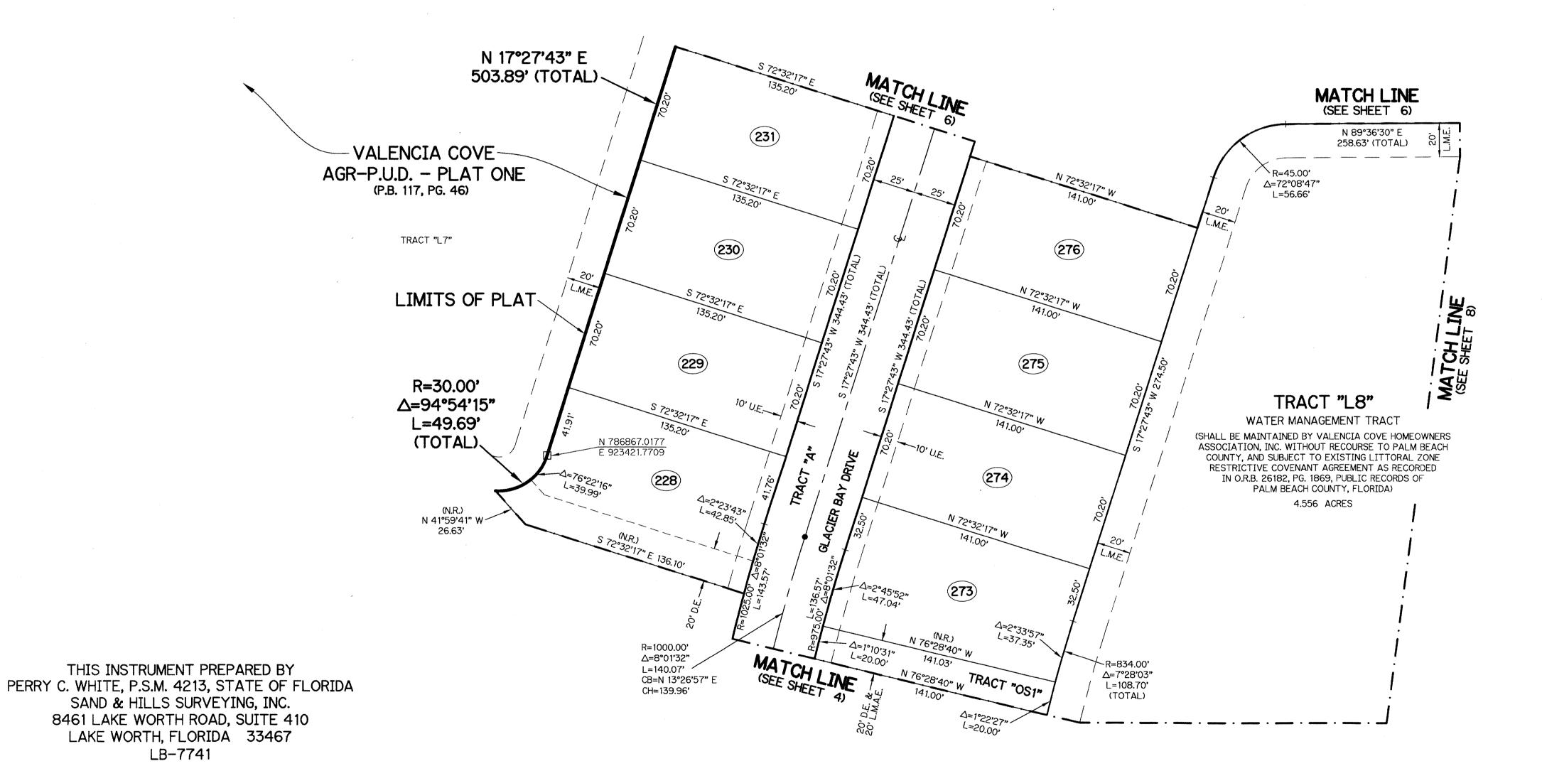
COORDINATES SHOWN ARE GRID COORDINATES DATUM = NAD 83 (1990 ADJUSTMENT) ZONE = FLORIDA EAST ZONE LINEAR UNIT = U.S. SURVEY FEET COORDINATE SYSTEM = 1983 STATE PLANE TRANSVERSE MERCATOR PROJECTION ALL DISTANCES ARE GROUND SCALE FACTOR = 1.0000240 PLAT BEARING = GRID BEARING GROUND DISTANCE X SCALE FACTOR = GRID DISTANCE
